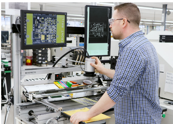
In-line timer-controlled interval display inspection
