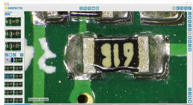
Resistor, focus stacked in INSPECTIS® ProX
